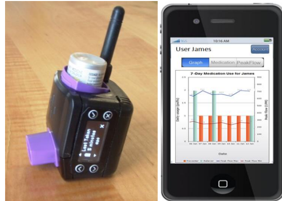
Figure 1: SmartInhaler device with on-board cell phone, and mobile application to view personal health data.
